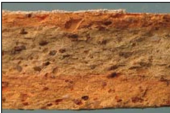
Figure 27: fabric of a red scaled grog mortarium found at Tongeren
